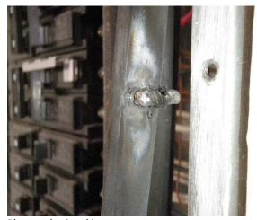
Photo submitted by: Brent Scott, Premier Home Inspection LLC \*\*Faceplate screw on a service panel that "welded" to the main conductor in the panel. It sparked when I was backing it out.
