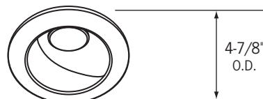
CTR2003-P Scoop Wall Wash All steel construction. (3) heat treated spring steel mounting clips. Black socket aiming bracket with screws (provided in carton).
