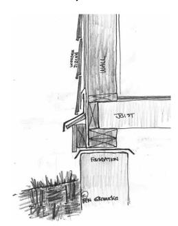
Clearance. Check the distance between the bottom of wood elements and grade. In locations that have little or no snow, the distance should be no less than
