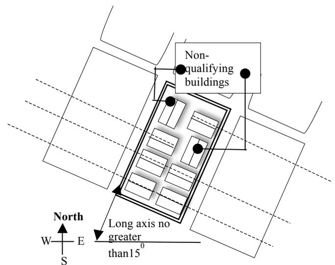
Figure 3. GIB: Solar orientation criterion for solar-oriented buildings (Congress, 2009, p. 97).
