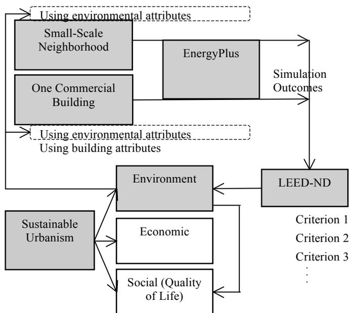
Figure 5. The proposed framework for urban scale energy efficiency regulation (defined attributes are remarked with grey boxes)
