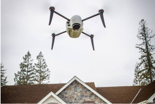
A Kesypry drone hovers over a home capture detailed images of the roof. PHOTO: KESPRY
