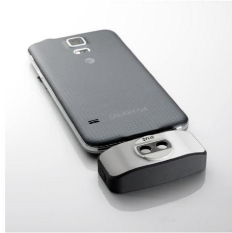
Figure 29.3 2015: FLIR One, an accessory to iPhone and Android mobile phones. Weight: 90 g (3.2 oz.).
